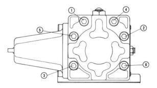
Notes: Bolt torquing must be done in sequence below to avoid damaging covers.
