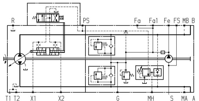
**Version with DA control valve and neutral position switch 1)**
